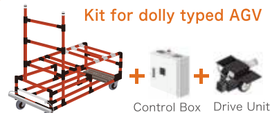
Forward & reverse 4WD Transportable weight : 1500kg L2660×W480×H290
